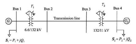
G1; 20 MVA, 6.6 kV, X = 0.10 pu
