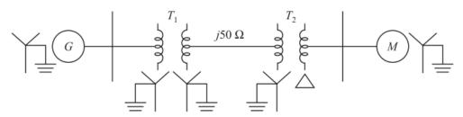
Neglect the resistance and use a base of 100 MVA, 220 kV in a 50  $\Omega$  line. The ratings of the generator, motor and transformers are as follows:
